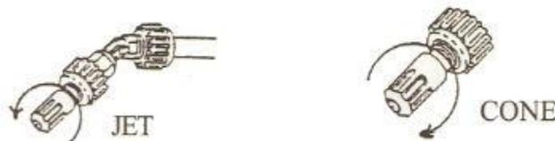
**CONE** -Turning the nozzle clockwise (toward the nozzle body) takes the nozzle to the CONE position. A wide variety of cone patterns are available as the nozzle is turned. Turn the nozzle as far as possible to the clockwise position and you will get a fine mist. This CONE is formed because as the nozzle is turned clockwise, it restricts the flow, thus putting out a smaller quantity of spray with finer water droplets.
